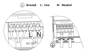
**Note:** The grounding wire shall be as thick as possible (cross-sectional area is not less than 4mm²). The grounding point shall be as close as possible to the all-in-one solar charge inverter. The shorter the grounding wire, the better.
